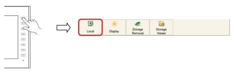
2) Current System program version and OS version can be checked on [System information] after switch to Local mode screen.
