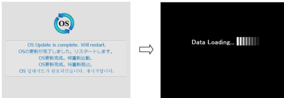
8) Switch back to Local mode screen by pressing [SYSTEM] button from [System menu] bar, and confirm System program version and OS version is updated.
